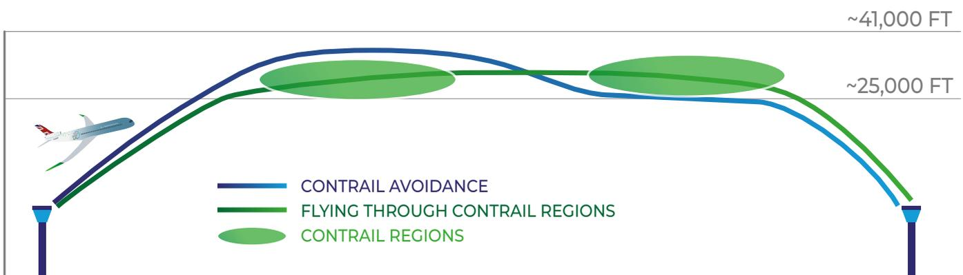
Figure 44 – Schematic representation of navigational contrail avoidance
