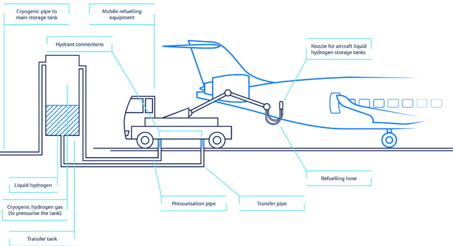
Figure 13 – Above ground transfer tank concept (Source: Jacobs)
