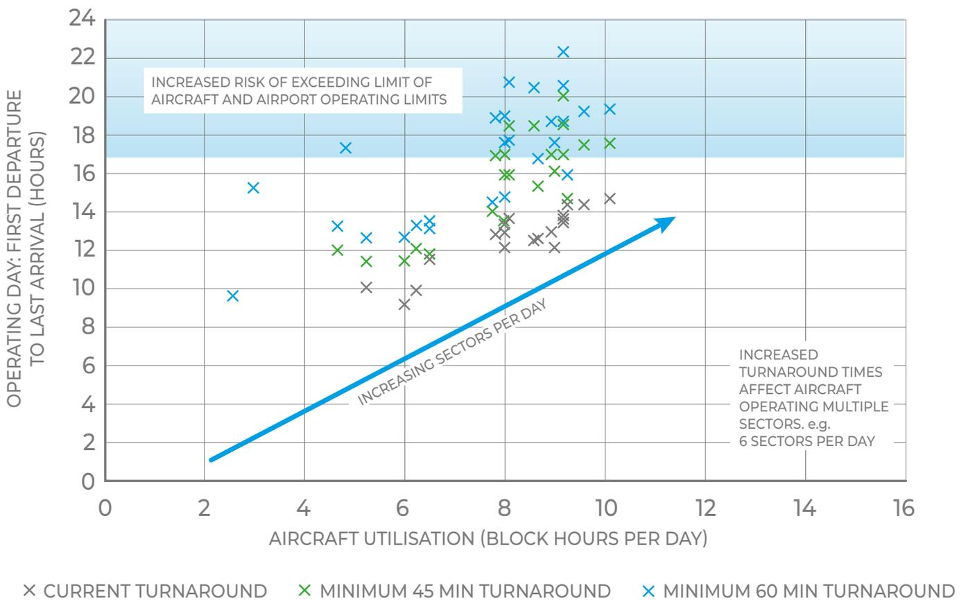
Figure 25 – Impact of longer turnaround times on typical low-cost airline schedule (Regional aircraft)
