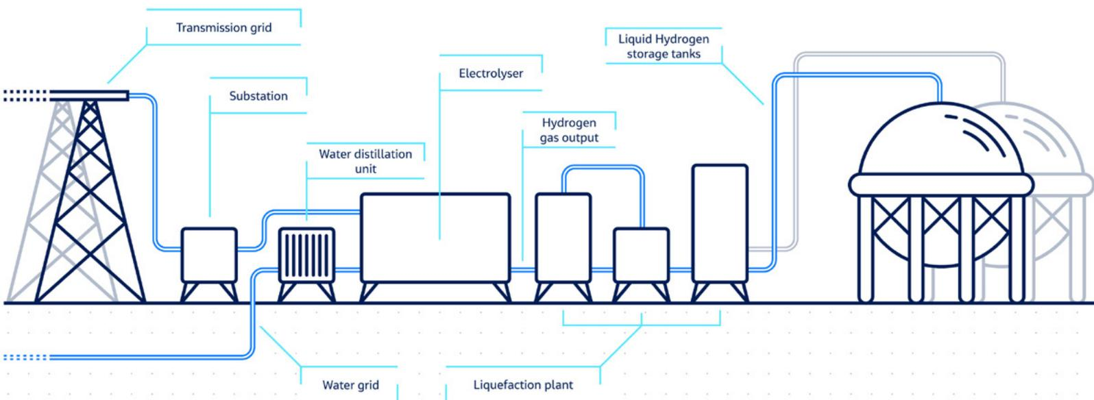
Figure 7 – Scenario 3 - On-site electrolysis and liquefaction (Source: Jacobs)
