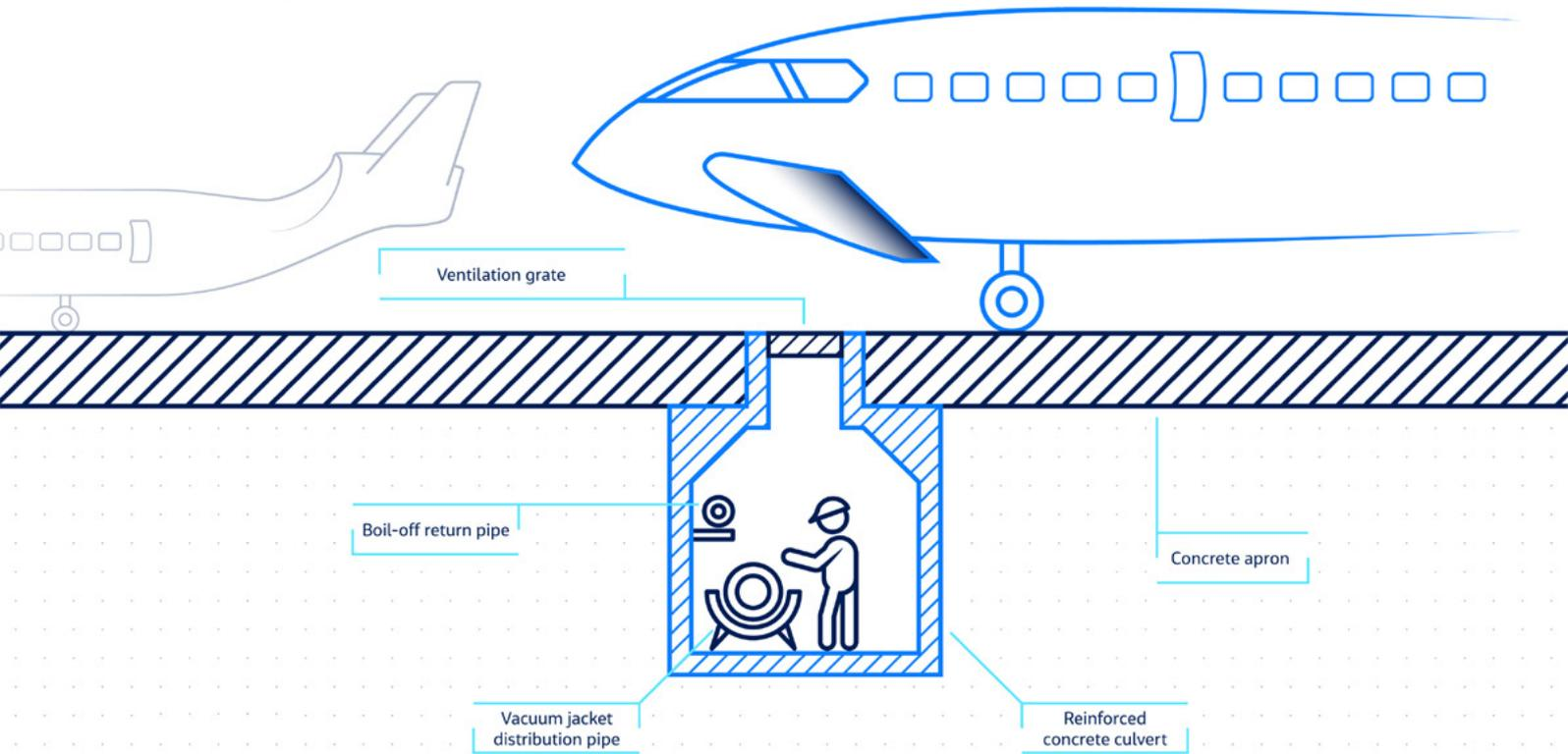
Figure 10 – Hydrant system concept (Source: Jacobs)
