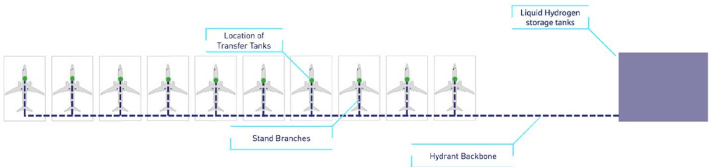
Figure 11 – Hydrogen hydrant concept layout
