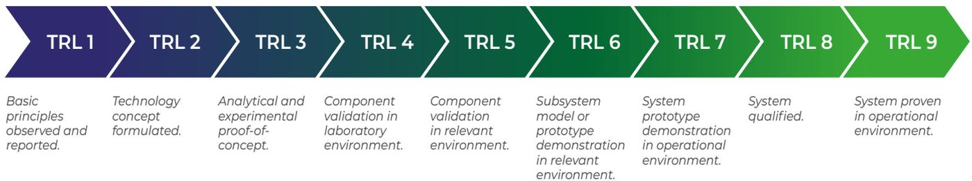
Figure 14 – Technology has been assessed against an adapted NASA Technology Readiness Level (TRL) scale.
