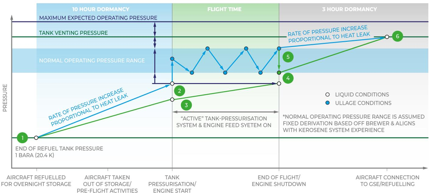
Figure 26 – Liquid hydrogen tank pressure variation during different flight cycle phases [8]
