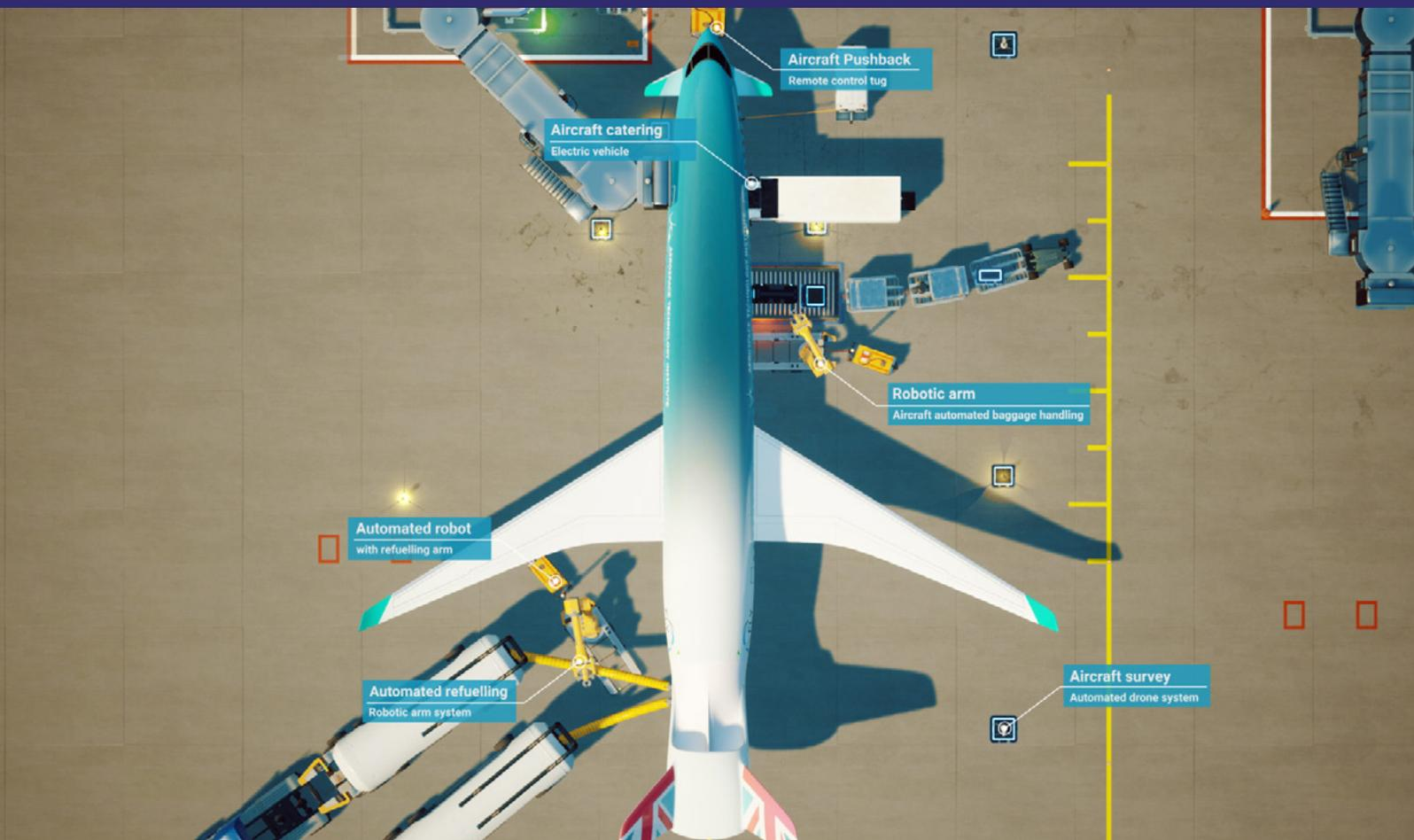
Figure 28 – Stand layout with GSE for FlyZero narrowbody concept refuelling with liquid hydrogen
