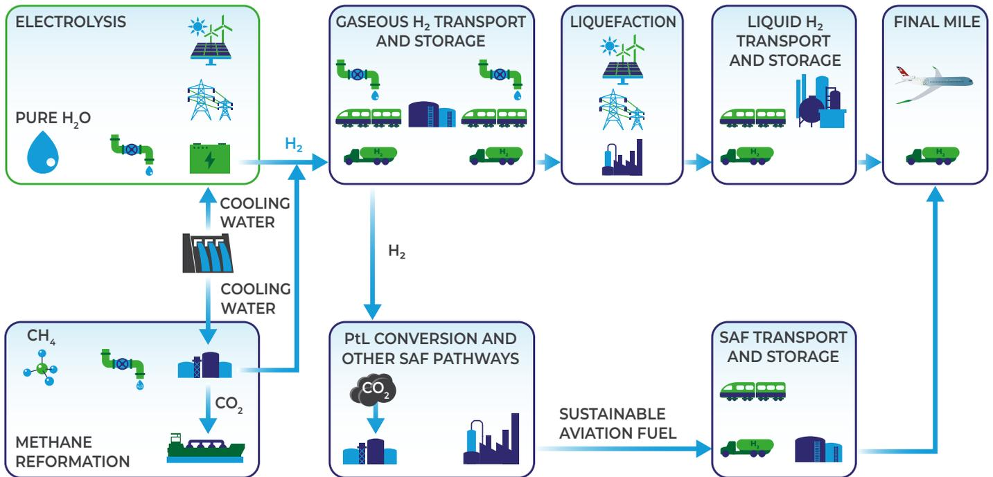
Figure 1 – Hydrogen and power to liquid (PtL) SAF generation pathways (Source: Arup)
