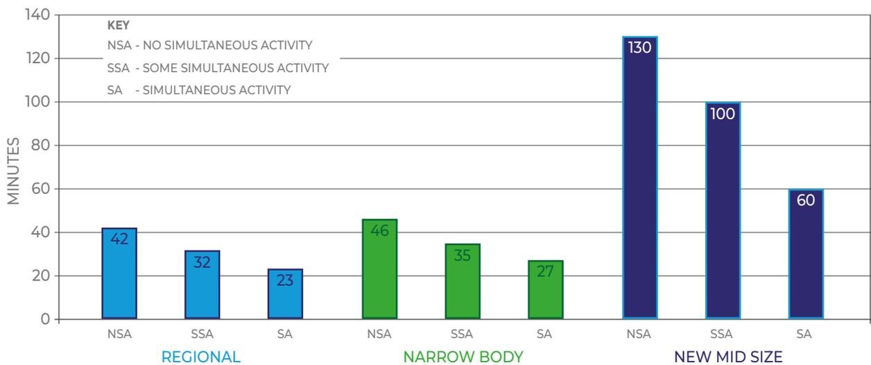
Figure 16 – Estimated turnaround times of FlyZero concept aircraft
