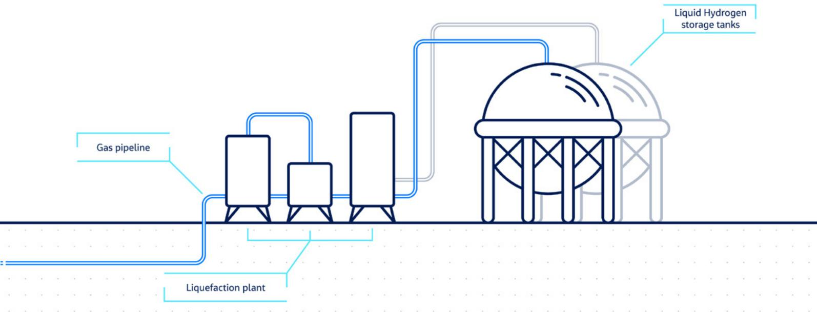
Figure 6 – Scenario 2 - Gaseous hydrogen pipeline supply to the airport with on-site liquefaction (Source: Jacobs)
