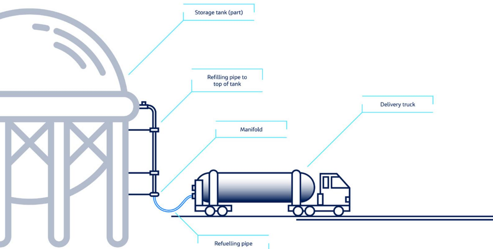
Figure 5 – Scenario 1 – Liquid hydrogen delivered to airport storage tanks (Source: Jacobs)
