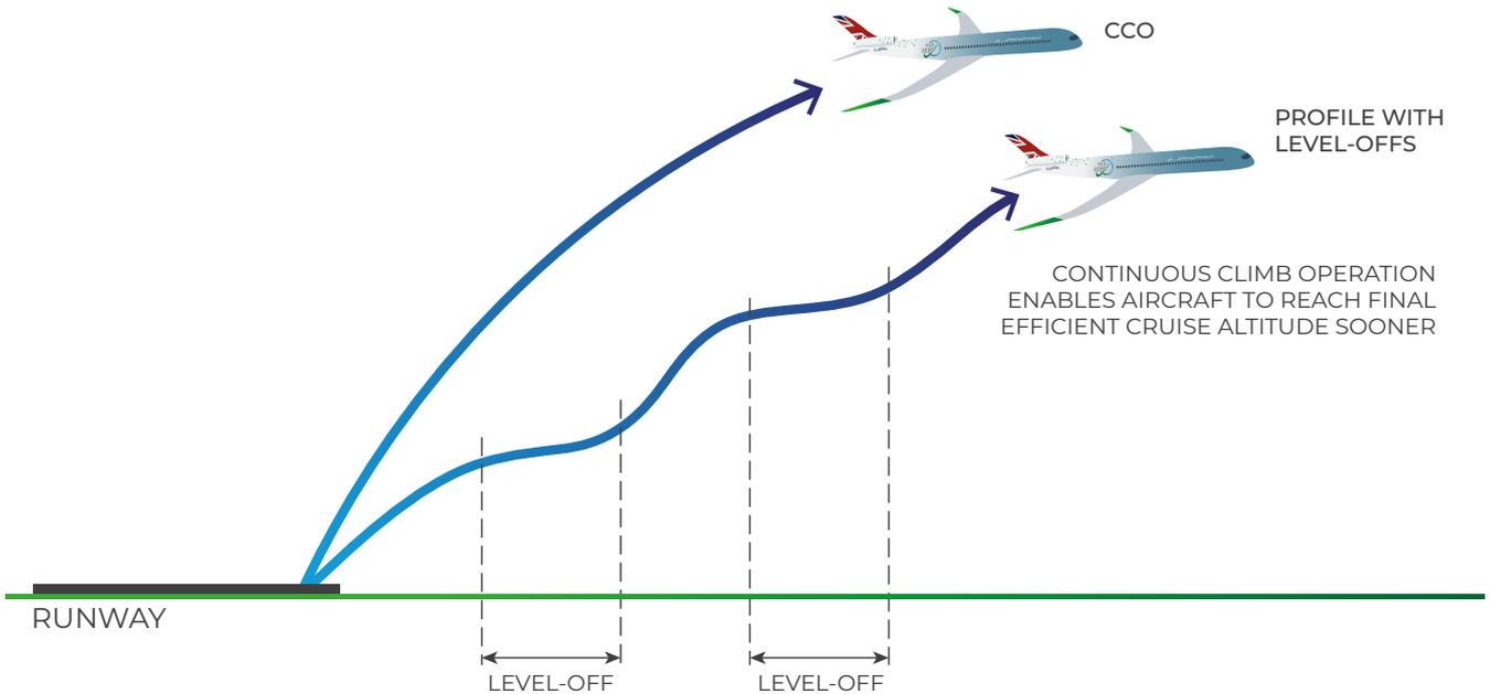
Figure 39 – Schematic representation of Continuous Climb Operation and comparison with conventional departure containing level segments
