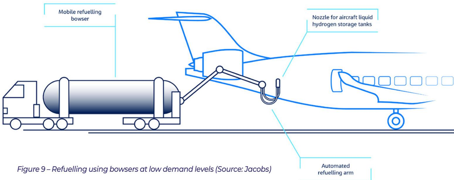
Figure 9 – Refuelling using bowser at low demand levels (Source: Jacobs)
