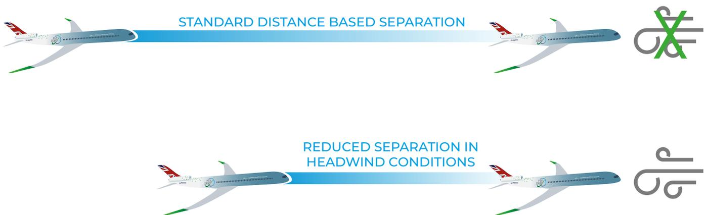
Figure 41 – Schematic representation of difference between distance-based separations and time-based separation in headwind conditions
