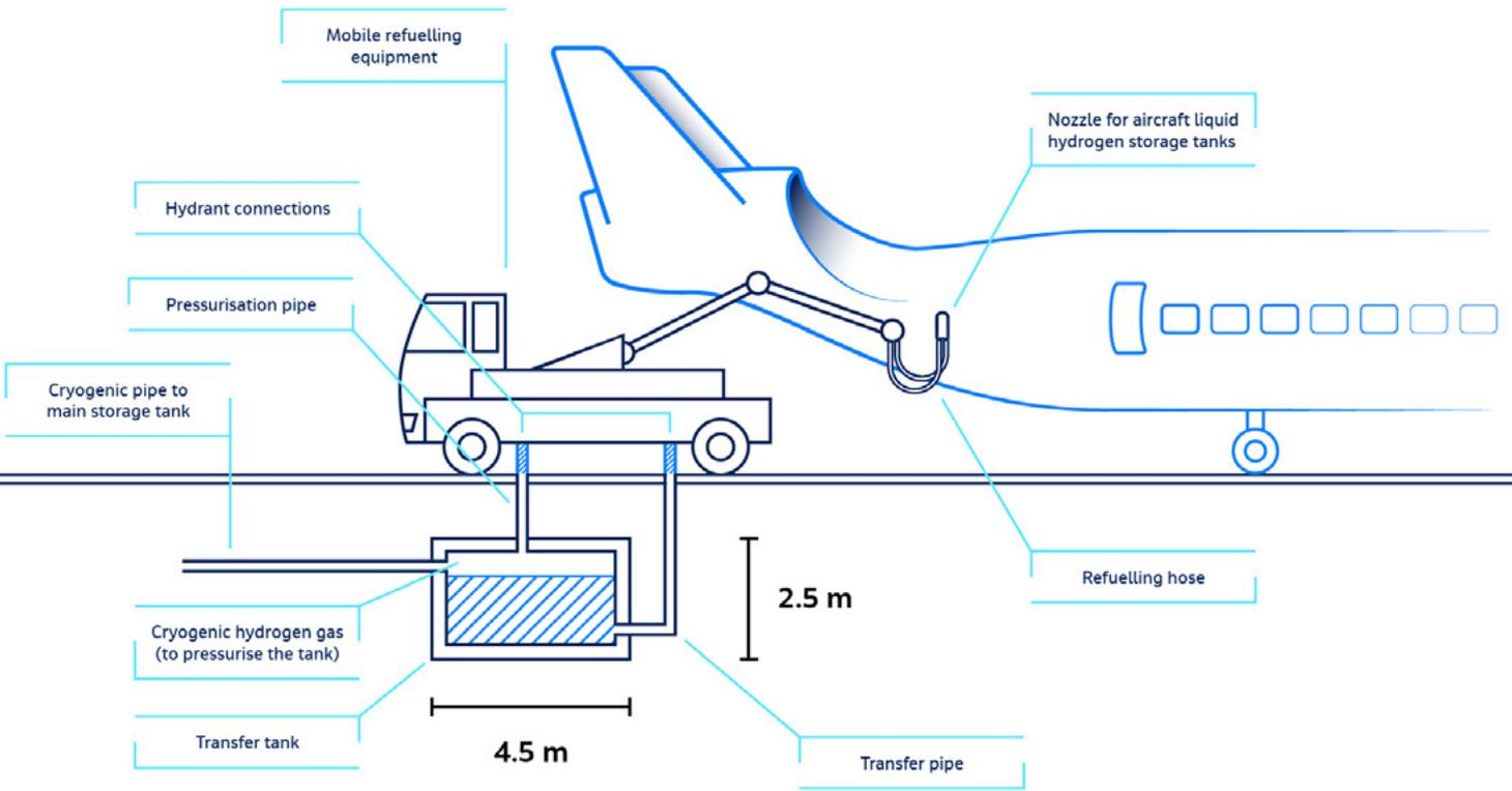
Figure 12 – Below ground transfer tank concept (Source: Jacobs)
