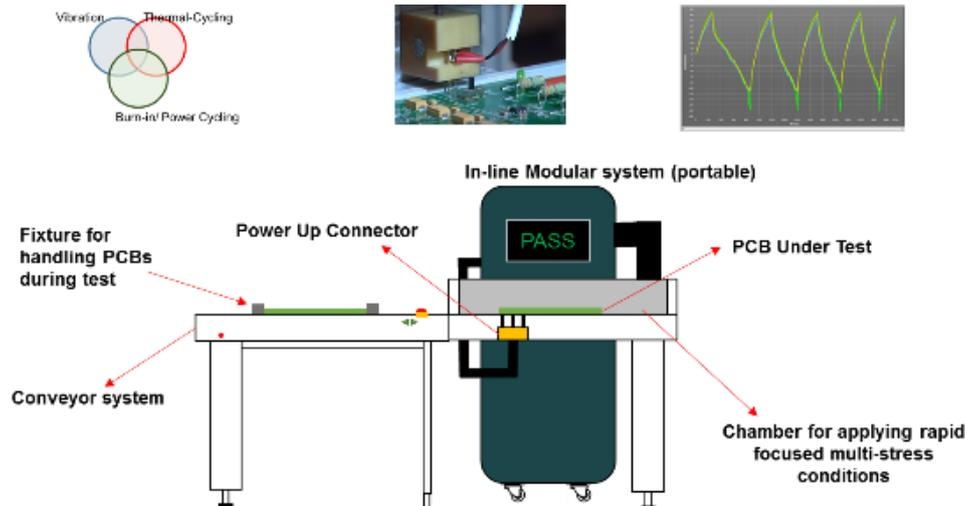
Fig. 8 in line stress screening concepts
