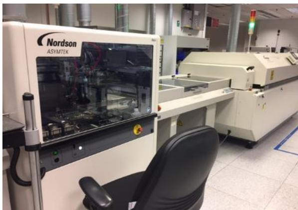
Fig. 7 Fully in line automated coating system
