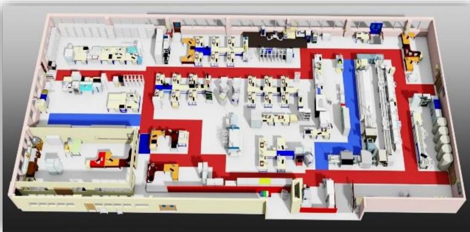
Fig. 3 3D model created of shop layout using OR3D mapping technology
