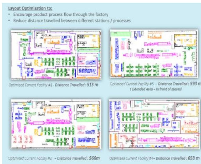
Fig. 4 Multiple layout iterations to optimise product / process flow.
