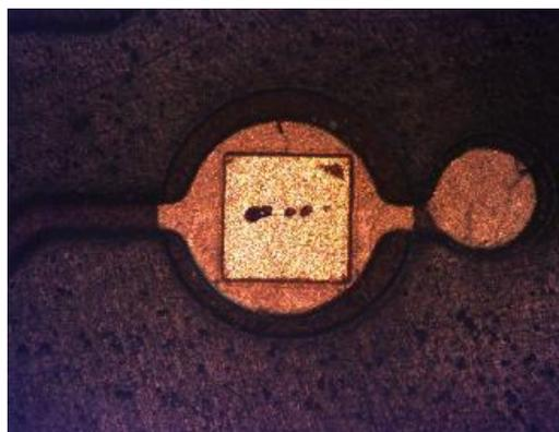
Fig. 9 Component pad with parylene removed by laser
