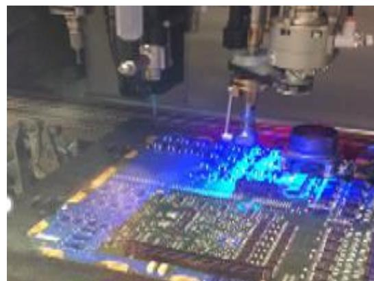
Fig. 6 Automated coating application
