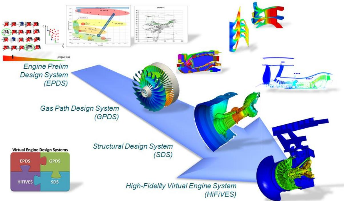
*Virtual Engine Design Systems (VEDS) to enable faster engineering simulation from conceptual to detailed product design*
