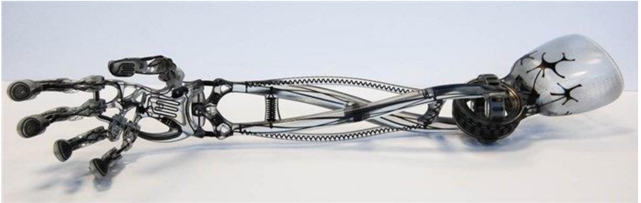
Multi-material bionic arm by 3D Printing Research Group at University of Nottingham. Source: www.nottingham.ac.uk/research/groups/3dprg/experience-our-group (2013)
