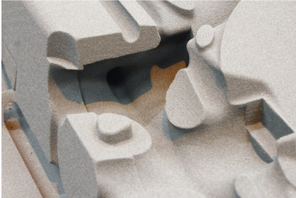
Additive Casting®, 3D printed sand moulds with geometrically challenging undercuts and cavities. Image courtesy of Enable Manufacturing Ltd.
