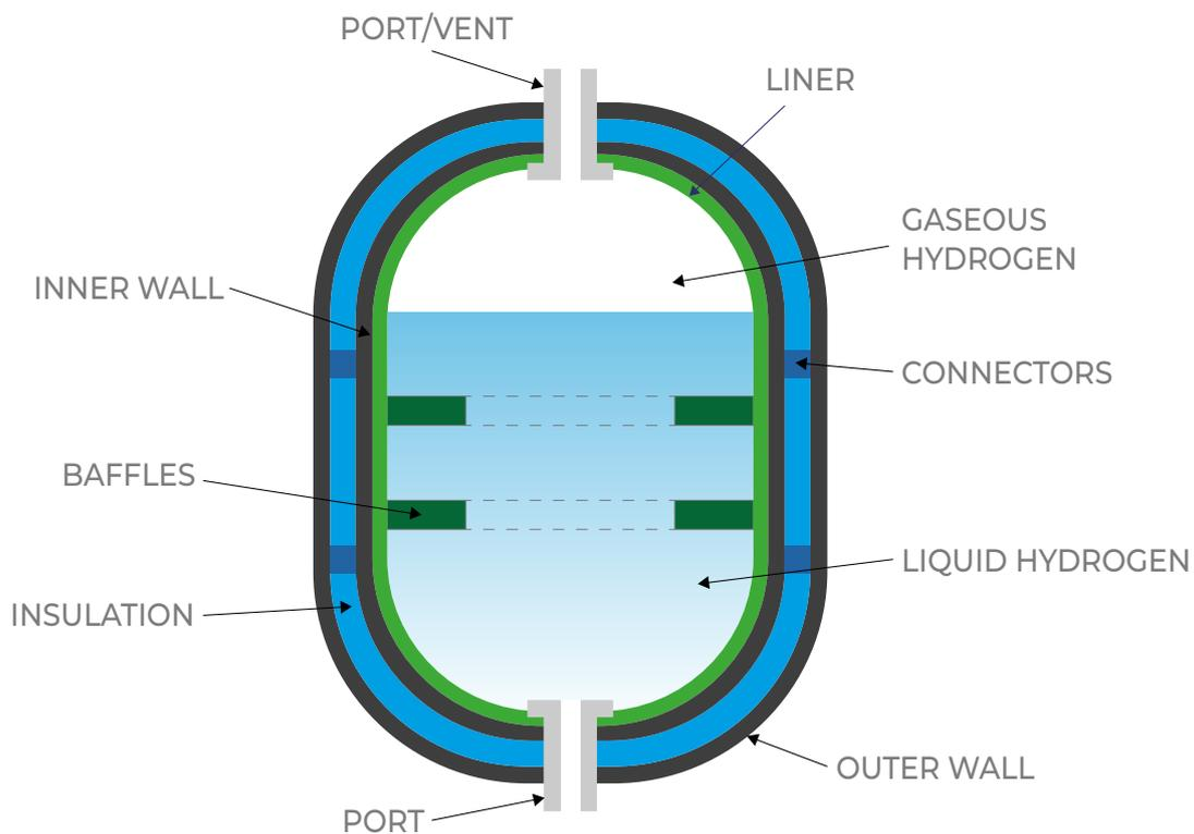
*Figure 8 – Schematic view of a double-walled cryogenic storage tank (Adapted from original image provided by NCC [18])*
