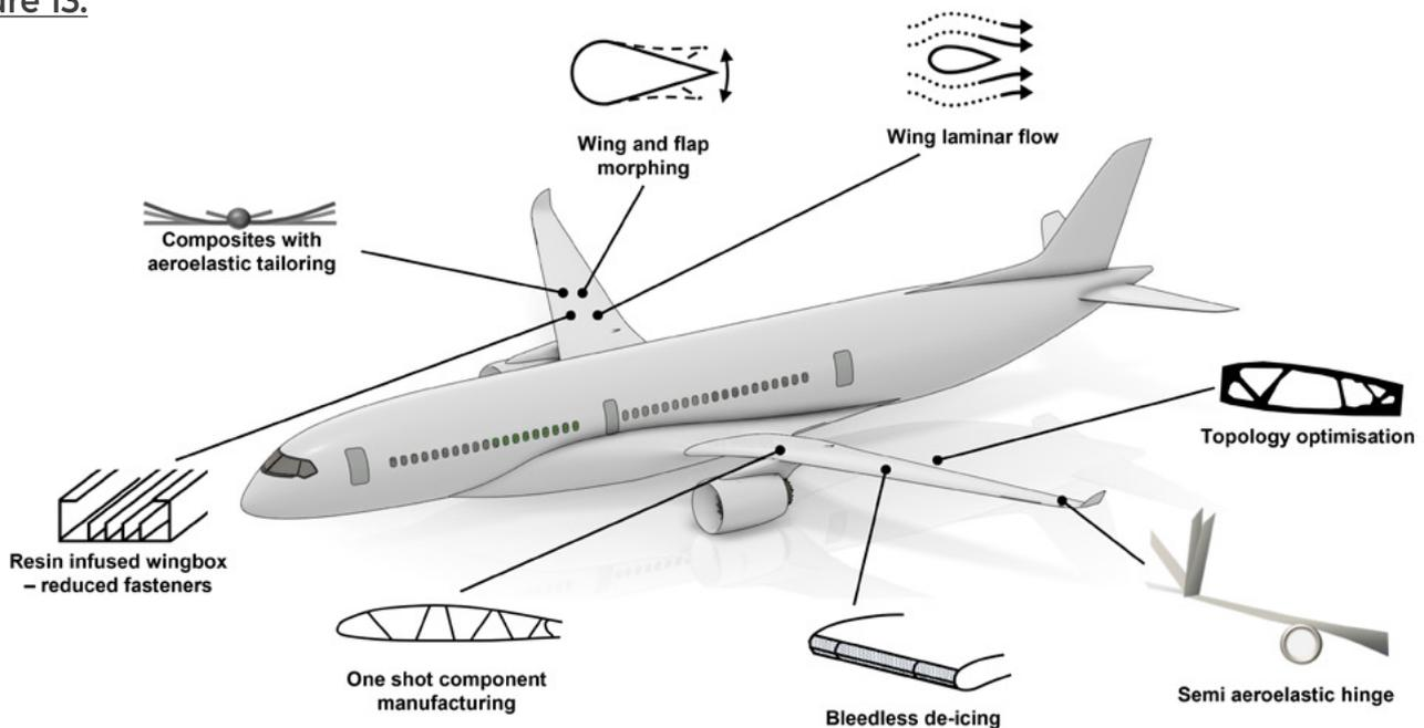
*Figure 13 – Potential technologies for future wings.*
