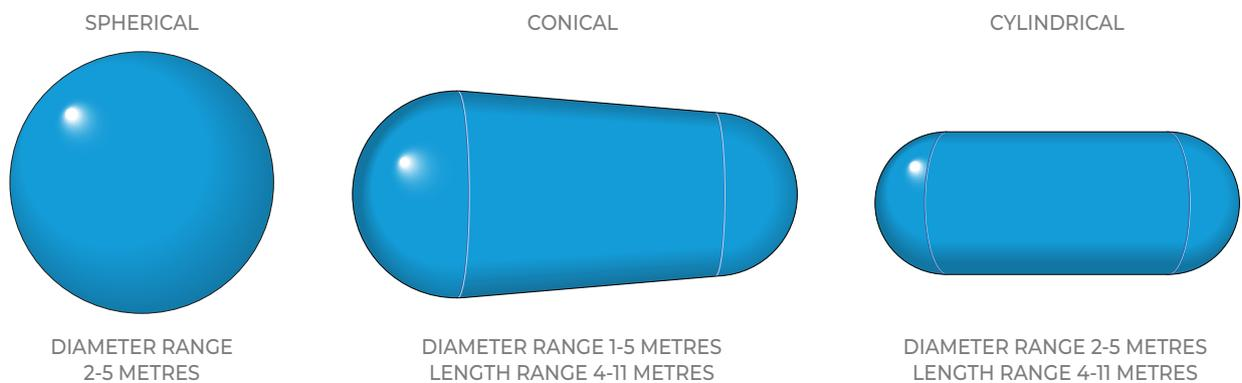
*Figure 7 – Potential shapes and expected size ranges for liquid hydrogen tanks, from FlyZero concepts*
