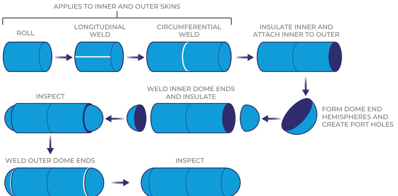
Figure 9 – Example manufacturing flow for a double-walled and insulated metallic tank
