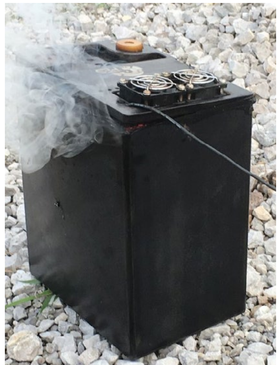
Figure 4 – Battery box manufactured with PS200 prepreg, using fire retardant, bio-based PFA resin. Undergoing fire test. (Image source © SHD Composite Materials Ltd)
