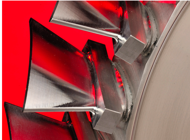
Linear friction welded compressor image courtesy of TWI.
