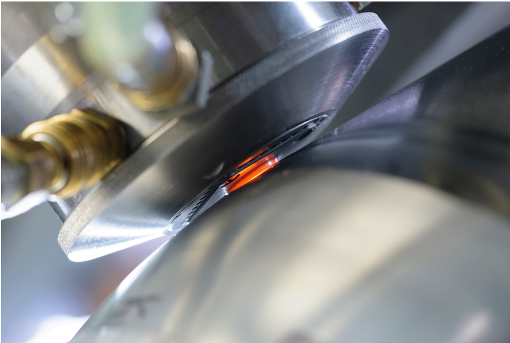
Friction stir welding, image courtesy of TWI.
