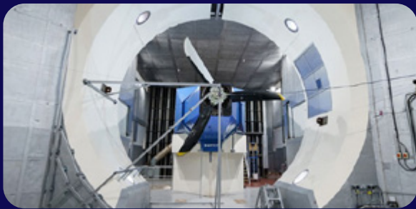
© Dowty. UK test capability includes Dowty's propeller spin-testing facility to assess structural and dynamic performance
