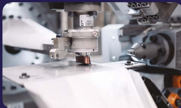
© Evolito. Automated copper coil winding machine supporting Evolito's scalable electric motor production.
