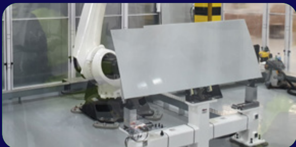
© Prestwick Aerosystems' A320 spoiler line utilises pioneering Resin Transfer Moulding (RTM) technology to deliver at rate and quality
